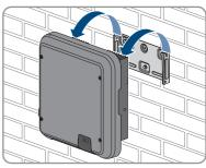
Unscrew the screws for fastening the wall mounting bracket and remove the wall mounting bracket.
