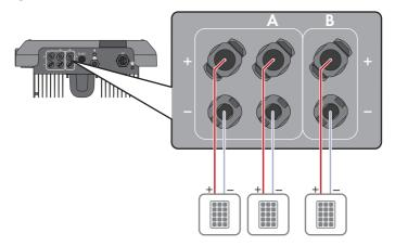
Figure 9: Connection overview for normal operation
