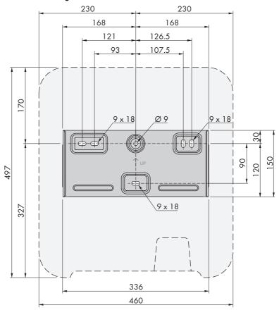
Figure 6: Position of the anchoring points(Dimensions in mm)
