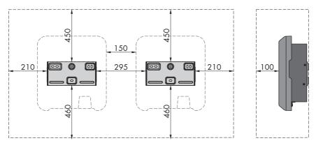
Figure 7: Recommended clearances(Dimensions in mm)
