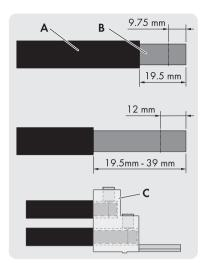
Figure 2.25 Connect to PV input
