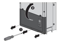
Figure 2.13 Loosen front screws and lift the cover
