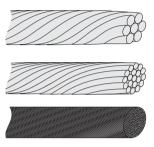
Figure 2.23 Cables with different conductors (from top to bottom): multi-strand, fine-strand and extra fine-strand
