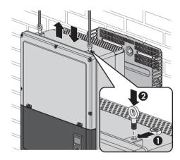
Figure 2.11 Attaching the lifting bolts and lifting the inverter
