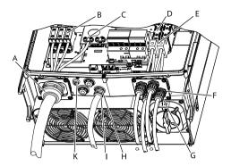
Figure 5.2 Overview of inverter with torque indications
