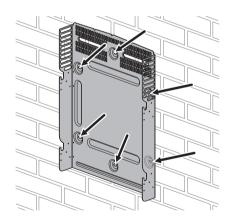
Figure 2.10 Mounting of the wall mounting bracket
