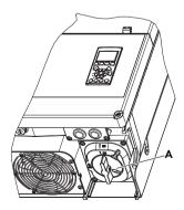
Figure 1: PV load-break switch
