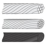
Figure 2.16 Cables with different conductors (from top to bottom): multi-strand, fine-strand and extra fine-strand
