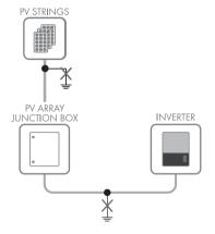
Figure 2.21 Do not connect PV to ground!
