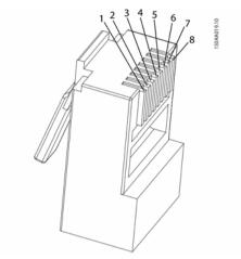
Table 5.4 Pin assignment of the RJ45 plug for Ethernet
