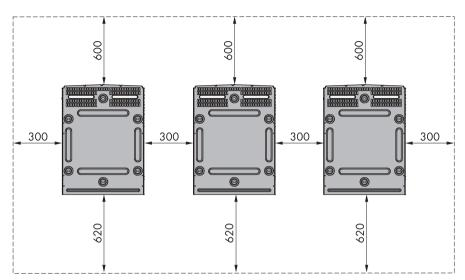
Figure 2.8 Safety clearances in mm
