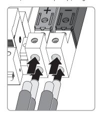
Figure 2.26 Connect to PV input
