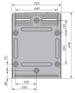
Figure 2.9 Dimensions of wall mounting bracket in mm
